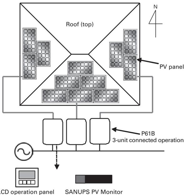
Fig. 5: An example of utilization as a string inverter
