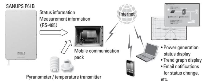
Fig. 7: A connection image of “Mobile Communication Pack”
