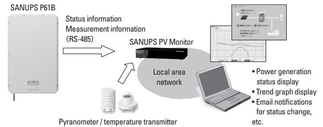
Fig. 6: Image of connection to the “SANUPS PV Monitor”
